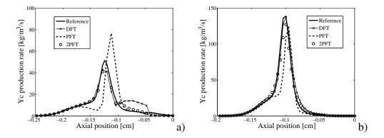
Figure 6: Production rates of the progress variable  $\dot{\omega}_{Y_c}$  for injection velocity a)  $v_g^f = v_l^f = 0.5~m/s$  and b)  $v_g^f = v_l^f = 1.0~m/s$  (continuous black line). Lines and symbols are the same as in Fig. 3.
