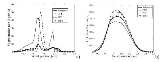
Figure 3: a) The production rate of the progress variable  $\dot{\omega}_{Y_c}$  and b) the CO mass fraction of the reference spray flame obtained with the detailed chemistry (black continous line) is compared to the a priori profiles for the three tabulated mechanisms: PFT premixed method (dashed gray line), DFT diffusion method (gray crosses), 2PFT technique (black circles).
