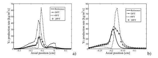
Figure 4: Production rates of the progress variable  $\dot{\omega}_{Y_c}$  for a)  $D_l^f=70~\mu m$  and b)  $D_l^f=140~\mu m$ . Lines and symbols are the same as in Fig. 3.
