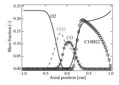
Figure 2: Species mass fraction profiles as a function of the axial position in the reference spray flame.
