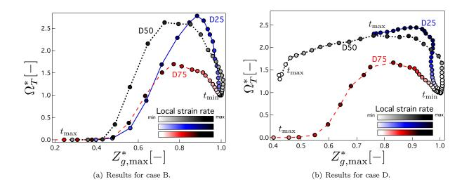
Figure 14: Flame quenching: Evolution of  $\Omega_T^*$  as a function of the maximum value of  $Z_g^*$  for Lf = 0.075 (blue), Lf = 0.3 (black), Lf = 0.675 (red), colored by the local strain rate. (For interpretation of the references to colour in this figure, the reader is referred to the web version of this article.)
