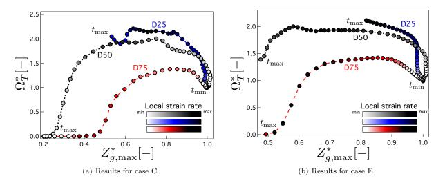
Figure 15: Fuel depletion: evolution of  $\Omega_T^*$  as a function of  $Z_{g,max}^*$  Lf = 0.075 (blue), Lf = 0.3 (black), Lf = 0.675(red), colored by the local strain rate. (For interpretation of the references to colour in this figure, the reader is referred to the web version of this article.)
