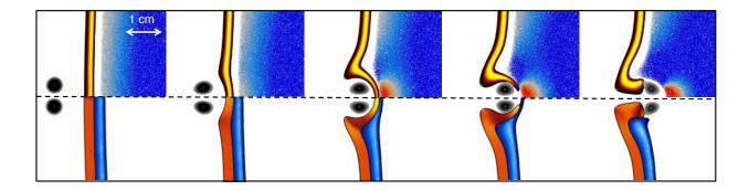
Figure 9: Temporal evolution of the spray flame-vortex interaction for the case with extinction due to strain rate (case B in Table 1 corresponding to  $r_v/\delta_L = 5/9$ ,  $\tilde{\Gamma} = 4$  and Lf = 0.3). Instantaneous fields at normalized time  $\tau = 0.0, 2.4, 2.8, 3.25, 3.5$  (from left to right). Legend is the same as in Fig. 6.
