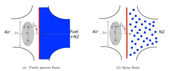
Figure 1: Schematic of the flame-vortex interaction for (a) purely gaseous flame and (b) spray flame: two counter-rotating vortices are superimposed to the initial steady-state solution of the counterflow flame. (For interpretation of the references to colour in this figure, the reader is referred to the web version of this article.)
