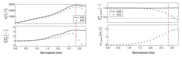
(a) Strain rate induced on the inner flame zone (top) and normalized mean heat release (bottom) as a function of normalized time.
