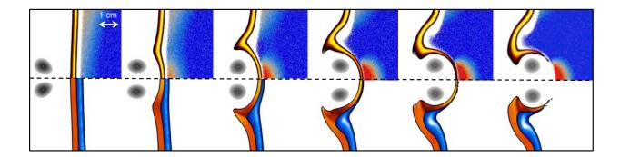
Figure 11: Temporal evolution of the spray-flame-vortex interaction for the case of extinction due to fuel depletion (case C in Table 1 corresponding to  $r_v/\delta_L = 10/9$ ,  $\tilde{\Gamma} = 2$  and Lf = 0.3). Instantaneous fields at normalized time  $\tau = 1.0, 2.25, 3.5, 4.75, 5.25, 5.35$  (from left to right). Legend is the same as in Fig. 6.
