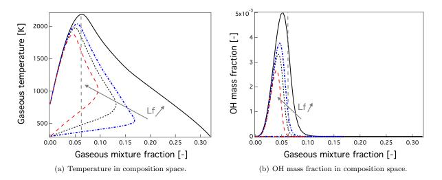
Figure 5: Structure of the steady gaseous (solid line) and spray flames (with increasing Lefebvre number Lf = 0.075, 0.3, 0.675at the centerline (y = 0 mm) in the  $Z_g$ -space. The vertical line indicates the location of stoichiometric mixture fraction. (For interpretation of the references to colour in this figure, the reader is referred to the web version of this article.)
