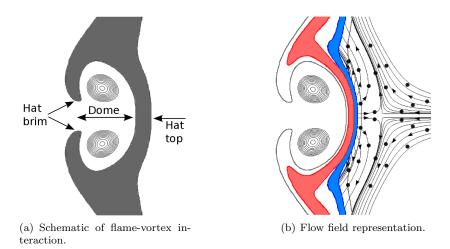
Figure 2: Qualitative features of a flame-vortex interaction [30]. The grey, red and blue regions in (b) identify the diffusion layer, the inner reaction zone and the evaporation zone, respectively. Streamlines are added to illustrate the droplet trajectories. (For interpretation of the references to colour in this figure, the reader is referred to the web version of this article.)
