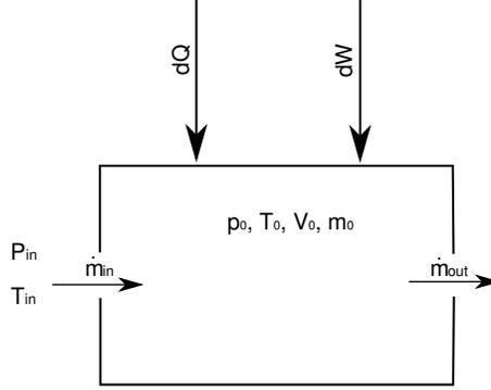
Fig. 2: Schematic of the control volume approach
