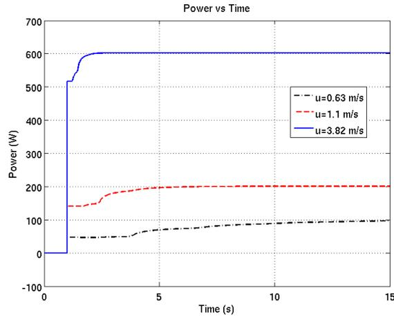
Fig. 5: Control Input for 3 different flow speeds
