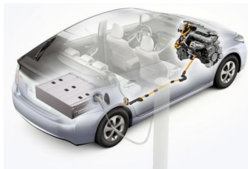
Fig. 10 Toyota Prius Plug-in Hybrid Electric Powertrain (Beissmann, 2011)
