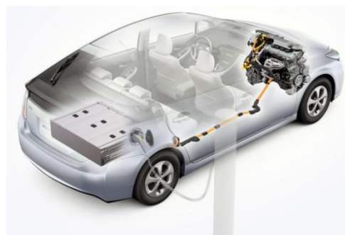
Fig. 10 Toyota Prius Plug-in Hybrid Electric Powertrain (Beissmann, 2011)
