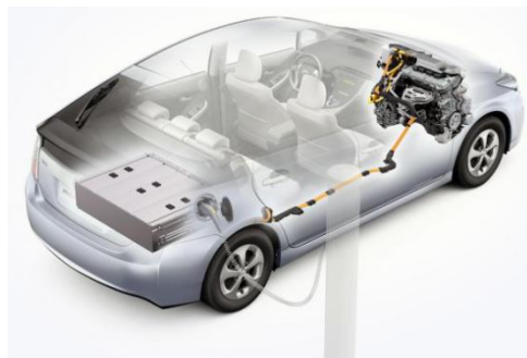
Fig. 10 Toyota Prius Plug-in Hybrid Electric Powertrain (Beissmann, 2011)
