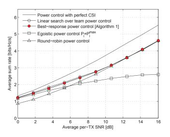
Fig. 1: Average sum-rate as a function of the maximum per-TX transmit power  $P^{\max}$  with K = 2.
