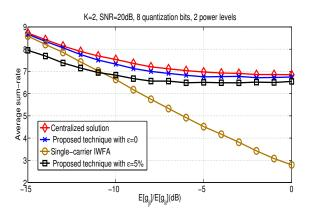
**Fig. 3.** Sum-rate against the interference level. The figure shows that by using the same feedback signal as the single-carrier IWFA during the exploration phase, it is possible to find a much better power vector for the exploitation phase.
