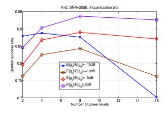
**Fig. 4.** Similar to how in conventional communication, a trade-off exists between the constellation size and bit error rate, here we have a trade-off between a higher number of power levels and the symbol success rate, which is plotted here.
