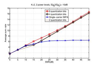
**Fig. 5.** The proposed technique outperforms the single-carrier IWFA in almost every case, with the exceptions being a small SNR or a high feedback quantization noise.
