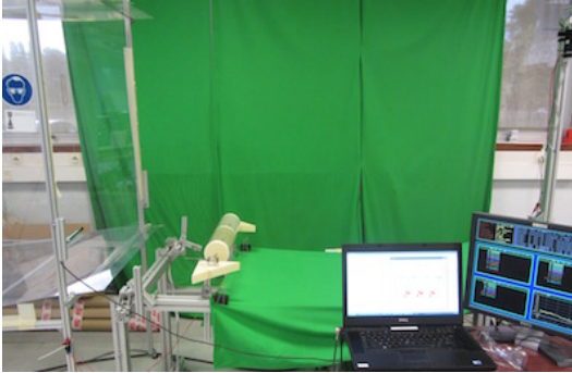
Fig. 3. The development and target computers for real-time experiments using Matlab/Simulink xPC target real-time toolbox.
