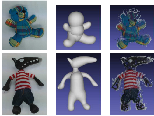
Figure 8. Comparison between reconstruction by multiview stereo (on the right), and the skeleton reconstruction (on the middle), with one of the origin images (on the left). We consider here textured objects, since multiview stereo can not reconstruct untextured objects. We can see here that both methods are complementary: multiview stereo gives details of the object, and skeleton based reconstruction gives a complete model with topology.
