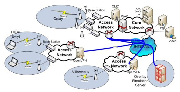
Fig. 9 Convergent underlay network composed of real POSEIDON's Alcatel-Lucent mobile WiMAX network and an overlay simulation platform [1].
