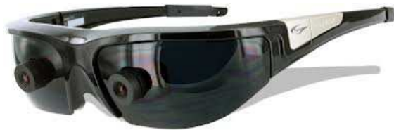
Figure 4: the Vuzix Wrap 920 AR glasses
