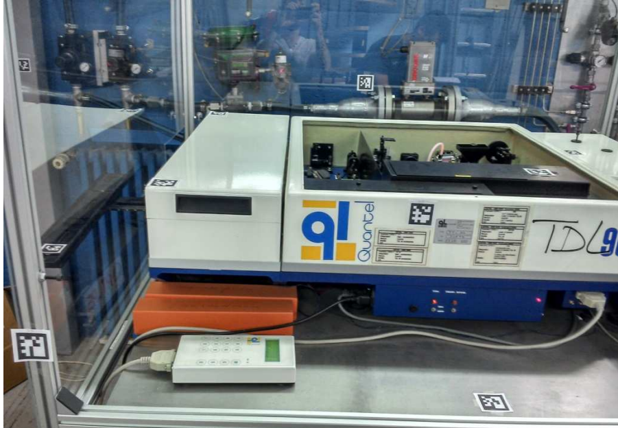
Figure 20: image of the markers stuck on a dye laser
