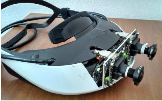
Figure 10: Cameras mounted on the Sony HMD
