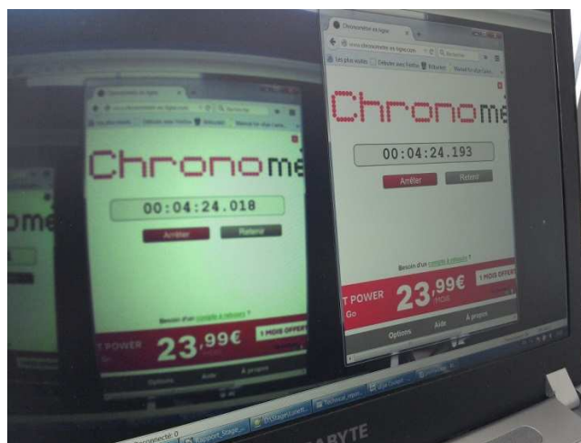
Figure 19: total lag measurement with screenshot of a timer
