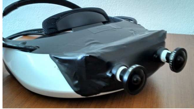
Figure 11: cameras mounted with protective plastic
