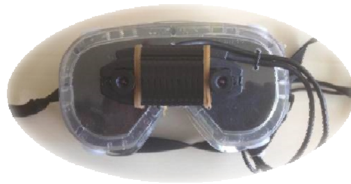
Figure 5: the Vuzix camera and displays mounted on a protective mask
