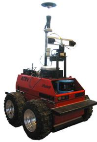
Fig. 8 LAAS-CNRS Dala robot with an ATRV base
