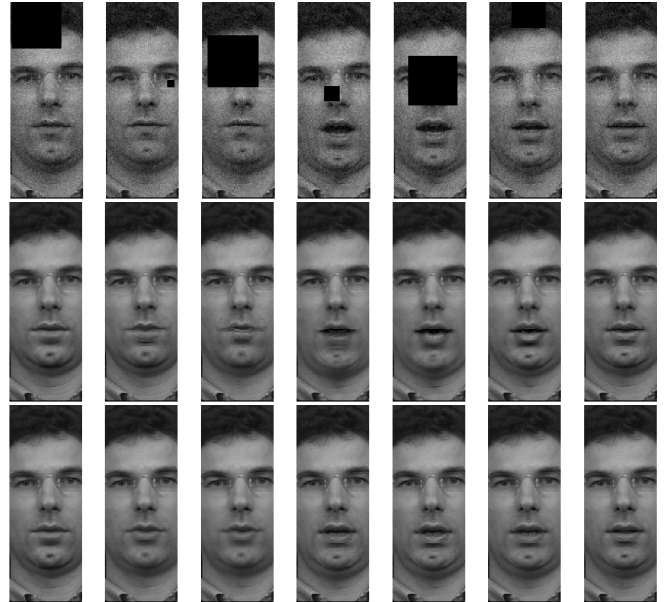
Fig. 5. face sequence. Algorithms are run conserving 99% of image energy for PCA. The first images are observations, second row shows results of AR model based data assimilation algorithm and the third row highlights results of our data-driven model based algorithm.
