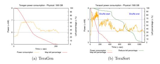
Figure 5: TeraGen and TeraSort percentage of remaining map/reduce and power consumption with collocated data and compute layers on servers for 500 GB. Map and reduce completion correlates with decrease in power consumption.
