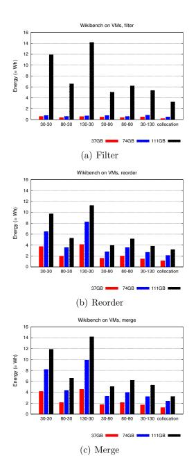
Figure 4: Hadoop Wikipedia data processing energy for three data-intensive operations with separated data and compute services on VMs. Filter benefits from more data nodes until the I/O becomes the bottleneck at ratio 130-30. Reorder and merge benefit from having more compute nodes.
