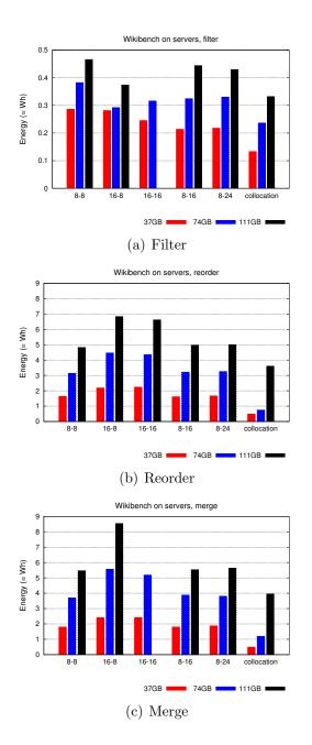
Figure 3: Hadoop Wikipedia data processing energy for three data-intensive operations with separated data and compute services on servers. The filter operation benefits from more data nodes. Reorder and merge benefit from more compute nodes.
