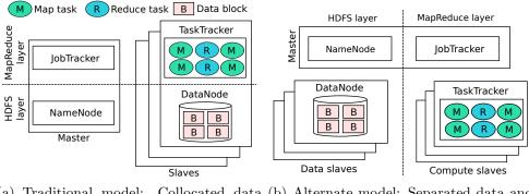
(a) Traditional model: Collocated data (b) Alternate model: Separated data and and compute compute
