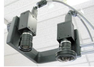
Fig. 5. Mixed stereo sensor in a second configuration with the fisheye camera on the right side of the image and the perspective on the left side.
