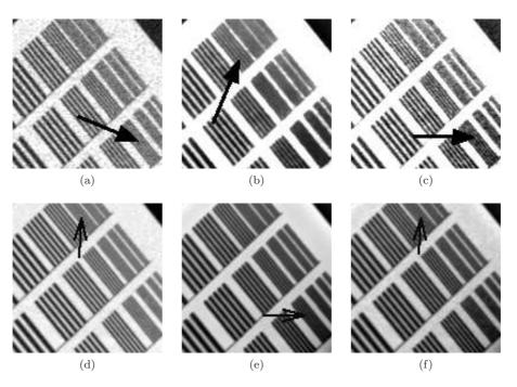
Figure 6: Resolution grid of the phantom: top row =  $10\mu Gy$  and bottom row =  $215\mu Gy$ ; columns from left to right = IN, DE and LNCE. For each example, the arrows indicate the finest, clearly visible, set of lines.
