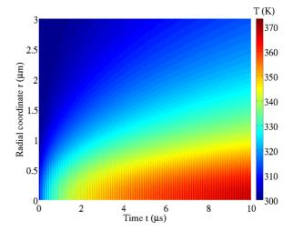
FIG. 3. Time evolution of radial distribution of the glass temperature T(r,t) during laser heating process:  $E_0=150$  nJ,  $\nu=10$  MHz,  $\tau_p=470$  fs,  $a_0=1.2$   $\mu$ m,  $L_z=10$   $\mu$ m, and full time 10  $\mu$ s corresponds to the 100 laser pulses.
