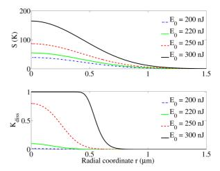
FIG. 5. (Top) Source terms in the heat diffusion equation S(r) for input laser pulse energies  $E_0 = 200, 220, 250,$  and 300 nJ, calculated according to Eq. (13). (Bottom) Corresponding dissociation function  $K_{diss}(r)$  calculated according to Eq. (29). Dissociation function parameters are  $S_0 = 80, N = 6$ .
