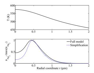
FIG. 4. (Top) Radial distribution of lattice temperature. (Bottom) Radial distribution of the silver cluster concentration  $n_{\text{Ag}_2^+}$ . Full model (black solid line) and simplified model (blue dashed line) predictions are provided. The input laser pulse energy is  $E_0 = 200 \, \text{nJ}$ , number of pulses is Np = 1000. Dissociation function parameters are:  $S_0 = 80$ , N = 6.
