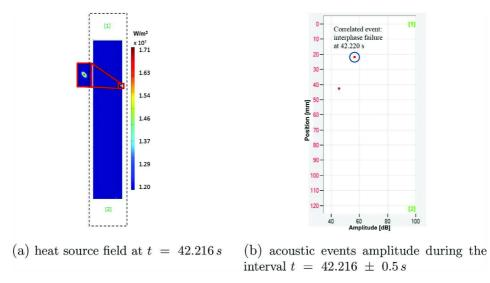
Fig. 8. Analysis of the correlation between high heat source and acoustic amplitude (90° tensile test).
