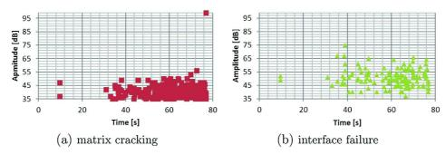
Fig. 3. Clustering results according to amplitude and time and related to identified damage mechanisms for the 90° tensile test (k-means algorithm, 3 descriptors, 2 classes).
