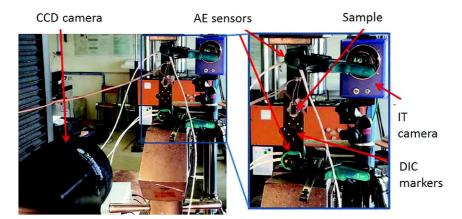
Fig. 1. Experimental setup.
