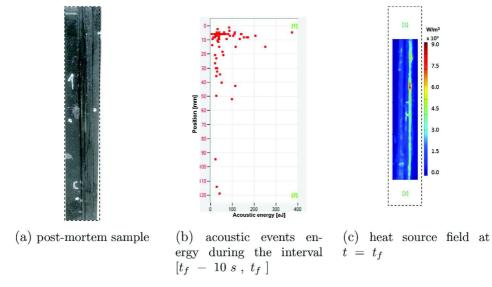
**Fig. 7.** Analysis of the correlation between AE and IT around breaking time  $t_f$  (0° tensile test).
