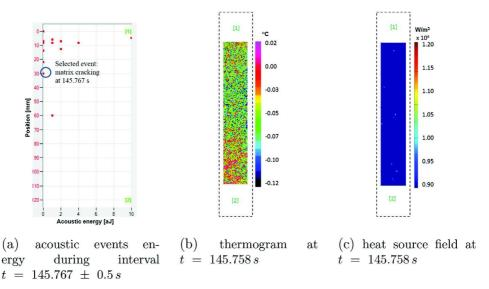
**Fig. 4.** Analysis of the correlation between low acoustic energy and heat source (0° tensile test). Numbers in brackets correspond to sensors with sensor [1] (respectively [2]) positioned on the top (resp. bottom) of the specimen; vertical position of the figures fulfils the studied areas of the sample.
