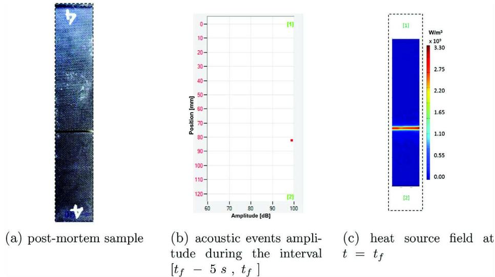
Fig. 9. Analysis of the correlation between AE and IT around breaking time  $t_f$  (90° tensile test).
