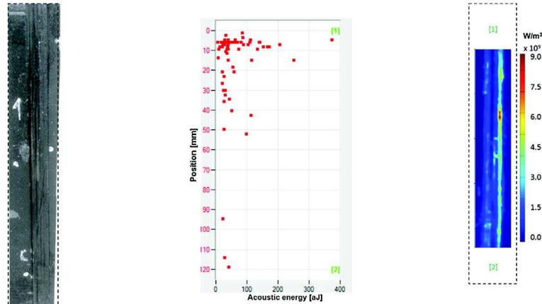
(a) post-mortem sample (b) acoustic events energy during the interval  $[t_f - 10$  s ,  $t_f$  ] (c) heat source field at  $t = t_f$
