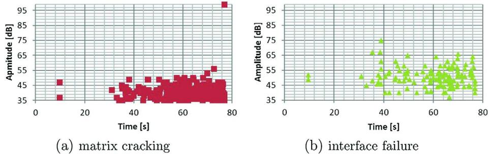
Fig. 3. Clustering results according to amplitude and time and related to identified damage mechanisms for the 90° tensile test (k-means algorithm, 3 descriptors, 2 classes).
