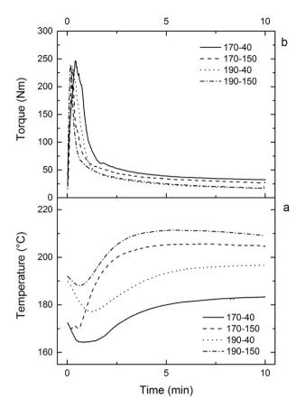
**Fig. 3.** Evolution of (a) torque and (b) polymer temperature of undried PLA for different batch mixing parameters: mixing temperature (170 or 190  $^{\circ}$ C) — rotor speed (40 or 150 rpm).
