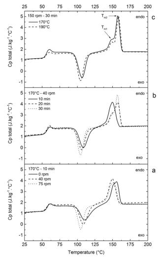
**Fig. 9.** Influence of processing parameters on heat capacity of PLA: (a) rotor speed (0, 40 and 75 rpm) at 170  $^{\circ}$ C for 10 min, (b) time (10, 20 and 30 min) at 170  $^{\circ}$ C and 40 rpm and (c) temperature (170 and 190  $^{\circ}$ C) at 150 rpm for 30 min.
