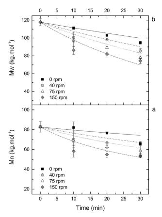
**Fig. 5.** Influence of rotor speed and mixing time at 170  $^{\circ}$ C on (a) number-average and (b) weight-average molar masses. Lines correspond to the simulation using the steady-state temperature and the constants determined for undried PLA (0 rpm: solid, 40 rpm: dashed, 75 rpm: doted, 150 rpm: dash-dot).
