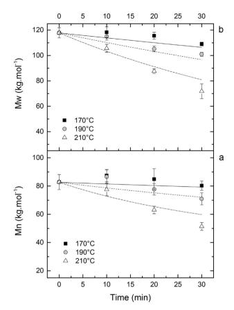
**Fig. 2.** Influence of time and temperature during processing by thermo-compression on (a) number-average and (b) weight-average molar masses for dried PLA. Lines represent the simulations (170 °C: solid, 190 °C: dashed, 210 °C: dash-dot).
