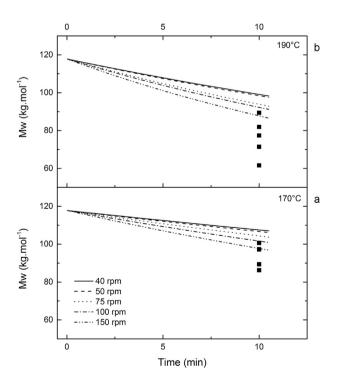
**Fig. 6.** Influence of set temperature ((a) at 170  $^{\circ}$ C and (b) at 190  $^{\circ}$ C) on weight-average molar masses for a mixing time of 10 min and various rotor speeds. Lines represent the corresponding simulations.
