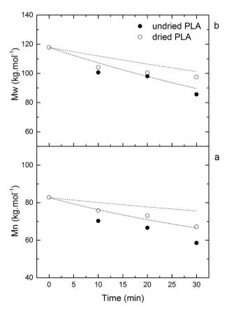
**Fig. 8.** Influence of drying on (a) number-average and (b) weight-average molar masses at 170  $^{\circ}$ C and 40 rpm. Lines represent the simulations using the steady-state temperature and the constants determined for dried (dashed) and undried PLA (dash-dot).
