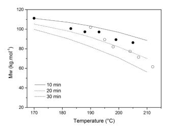
**Fig. 7.** Influence of steady-state temperature on weight-average molar mass after 10 min mixing at various set temperature (● 170 °C, fx1 190 °C) and various rotor speed. Lines represent the simulations for a mixing time of 10 (solid), 20 (dashed) and 30 min (dash-dot) at the corresponding steady-state temperature.
