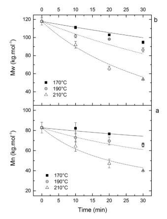
**Fig. 1.** Influence of time and temperature during processing by thermo-compression on (a) number-average and (b) weight-average molar masses for undried PLA. Lines represent the simulations (170 °C: solid, 190 °C: dashed, 210 °C: dash-dot).
