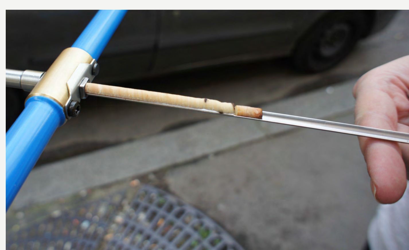
Tree core extraction with Pressler borer (March 2014)
