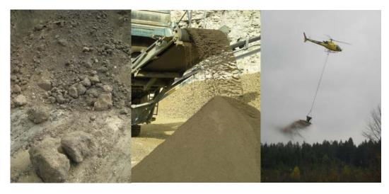
Figure 4. Tendency of wood – ash to generate clods because of its hydraulic properties (left), mechanical homogenization and mixing with Dolomite rock powder in limestone – works (centre), distribution of the mixture with helicopter (right)
