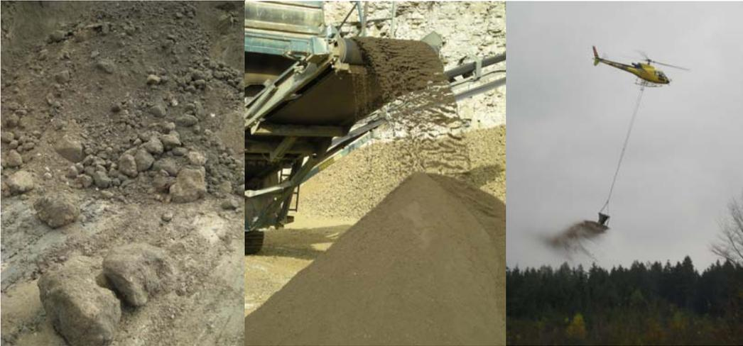
Figure 4. Tendency of wood – ash to generate clods because of its hydraulic properties (left), mechanical homogenization and mixing with Dolomite rock powder in limestone – works (centre), distribution of the mixture with helicopter (right)
