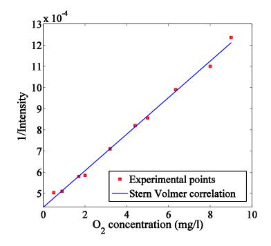
Figure 3. Calibration curve according to the Stern-Volmer equation
