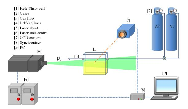
Figure 4. Experimental set-up for PLIF experiments
