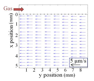
Figure 6. Velocity field in the liquid phase near the interface (Case 1) by PIV
