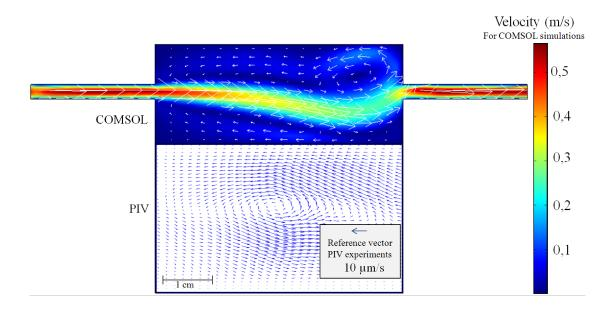
Figure 7. Velocity field (Case 1) in the liquid phase by PIV and in the gas phase
