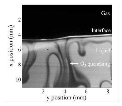
Figure 2. Fluorescence quenching by oxygen in the liquid phase
