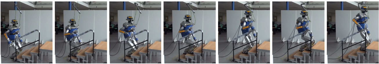
Fig. 8. HRP-2 in the stair climbing scenario.
