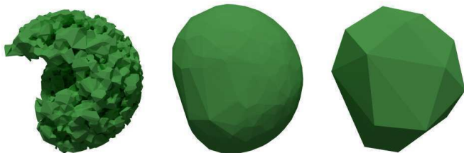
Fig. 15. Different approximations of the range of motion of the right arm of HRP-2. Left: non convex-hull, computed with the powercrust algorithm [37]. Middle: convex hull of the reachable workspace. Right: Simplified hull used in our experiments.
