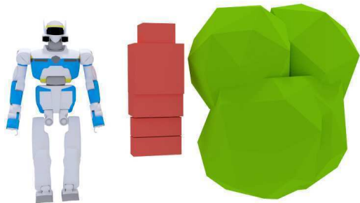
Fig. 14. The W volumes computed for HRP-2. The red shapes are W^0 . The green shapes represent the W^k .
