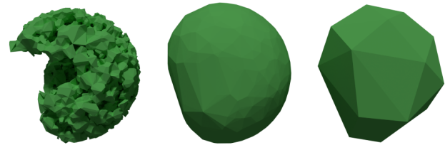
Figure 18. Different approximations of the range of motion of the right arm HRP-2. Left: non convex-hull, computed with the powercrust algorithm (Amenta et al. 2001). Middle: convex hull of the reachable workspace. Right: Simplified hull used in our experiments.
