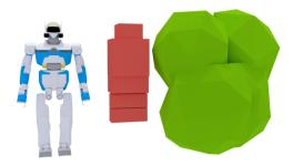
**Figure 17.** The W volumes computed for HRP-2. The red shapes are  $W^0$ . The green shapes represent the  $W^k$ .
