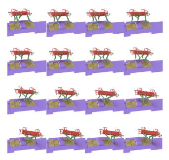
Figure 12. Robust crossing of rubbles by HyQ ( $b_0 > 20$ ).
