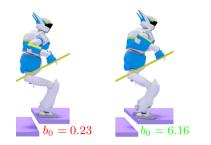
**Figure 9.** Evaluation of the robustness  $b_0$  of two contact configurations. Although in equilibrium, the left configuration is on the verge of slipping.
