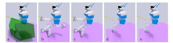
**Figure 2.** Generation of a contact configuration for the right leg of HRP-2. (a): Selection of reachable obstacles. (b): Entries of the limb samples database (with N = 4). (c): With a proximity query on the octree database, configurations too far from obstacles are eliminated. (d): The best candidate according to a user-defined heuristic h is chosen. (e): The final contact is achieved using inverse kinematics.
