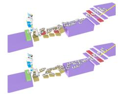
**Figure 15.** HRP-2 in the re-planning scenario. After the red step stones are removed, a new sequence of contacts is re-planned. Hand contacts are not presented here for readability.
