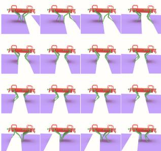
**Figure 14.** Crossing a hole contact sequence for HyQ  $(b_0 > 4)$ .
