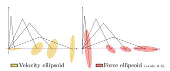
**Figure 6.** Examples of velocity and force ellipsoids for a manipulator composed of 2 dofs and 2 segments. Only the horizontal and vertical speeds are shown (not the rotation speeds), since it would require being able to draw in four dimensions.
