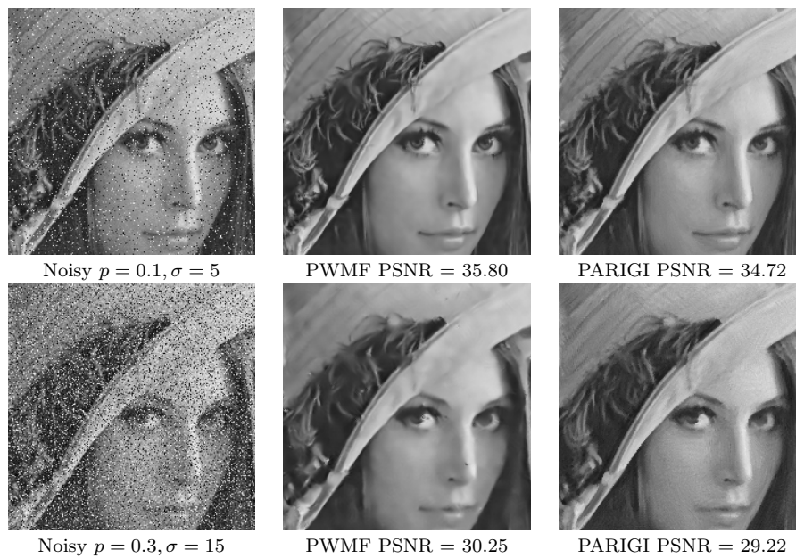
Fig. 5 Comparison of the performances of our filter PWMF and PARIGI [13] for removing mixed noise with Lena
