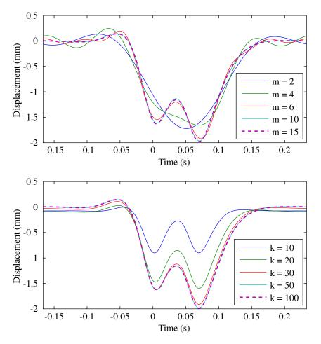
Figure 4: Displacement of a sleeper on a bilinear foundation by numerical method with different numbers of harmonics m (upper figure) and iterations k (lower figure)
