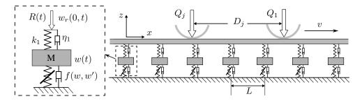
Figure 1: Periodically supported beam subjected to moving forces
