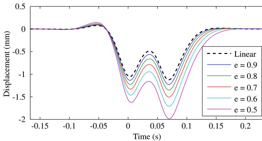
Figure 5: Displacement of a sleeper on bilinear foundations
