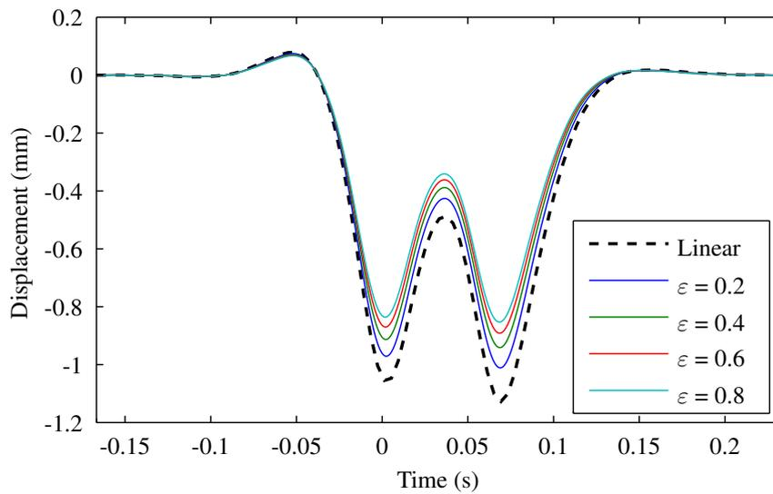
Figure 7: Displacement of a sleeper on nonlinear foundations
