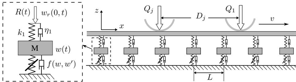
Figure 1: Periodically supported beam subjected to moving forces
