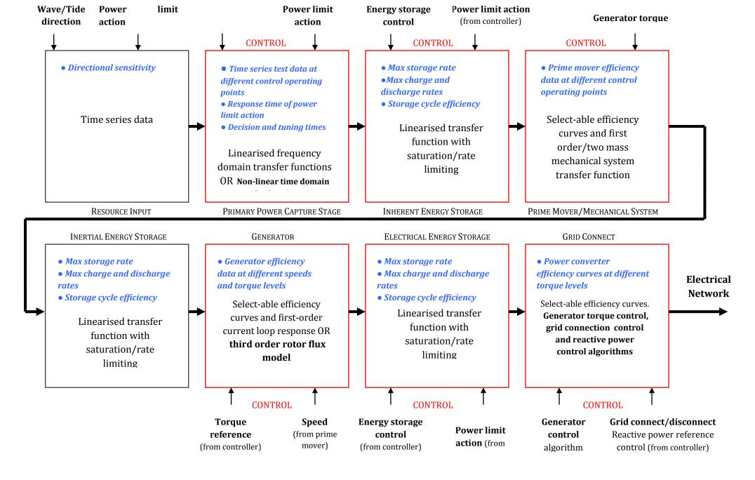
Figure 57: Dynamic Model Structure and Characterization Data
