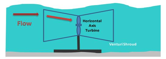
Figure 10: Venturi Effect Device Illustration
