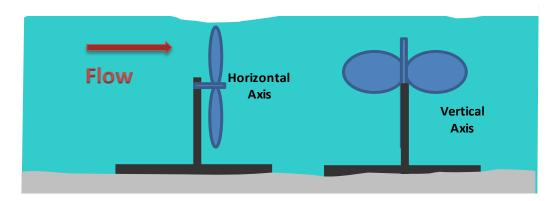
Figure 8: Horizontal and Vertical Axis Turbine Illustration
