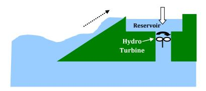
**Figure 7: Overtopping Device Illustration**
