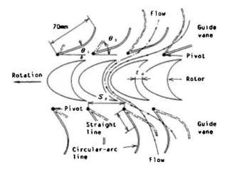
Figure 13: Impulse Turbine[27]
