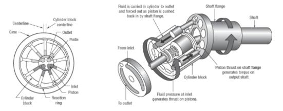
Figure 14: Radial Hydraulic Motor and Axial Hydraulic Motor [29]
