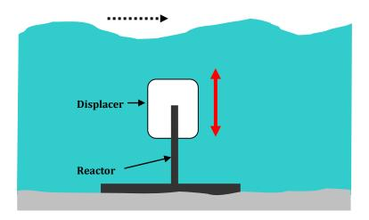
Figure 5: Submerged Pressure Differential Device Principle
