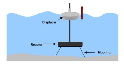
Figure 4: Point Absorber Illustration
