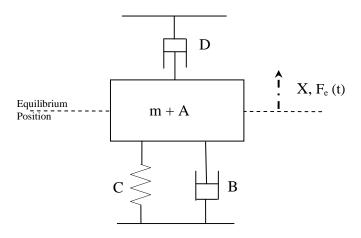
Figure 11: Spring-mass-damper System
