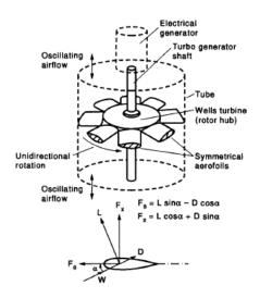
Figure 12: Wells Turbine and Blade Profile [25]
