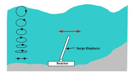
Figure 6: OWSC Schematic
