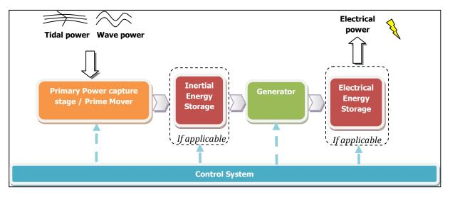
Figure 20: Colour Coded Model Reference (direct-drive systems)
