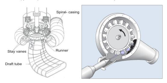
Figure 15: Reaction Turbine [31] and Hydro Impulse Turbine [32]
