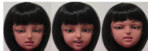
Figure 4: Synthesized Facial Expressions by ALICE Robot: Sadness, Happiness, and Anger (From Left to Right)
