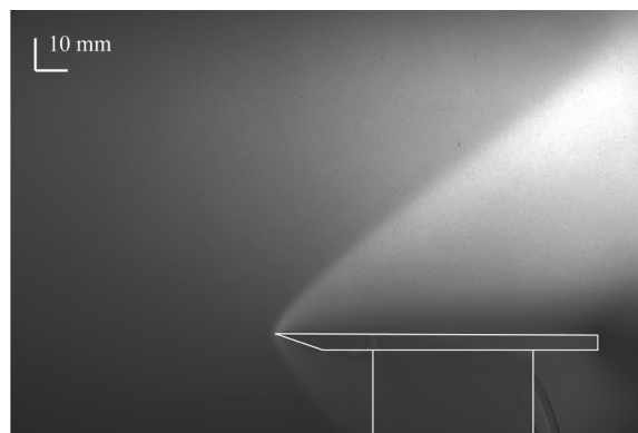
Figure 13 - Image of the natural flow field around the flat plate obtained with the glow-discharge flow visualization technique.
