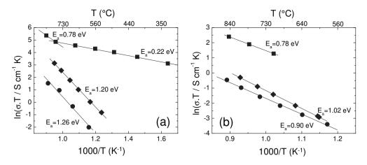
Fig. 5. Arrhenius plot of electrical conductivity for (♦) LBTM, (●) LBTMss, and (■) LBTCss measured (a) in Ar/H<sub>2</sub>(98/2) and (b) in air. Activation energy values (E<sub>a</sub>) were determined from the Arrhenius law.
