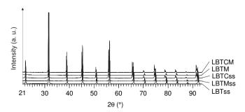
Fig. 2. XRD patterns of LBTss, LBTMss, LBTCss, LBTM, and LBTCM after synthesis in air and reduction at 900 °C for 48 h in Ar/ $H_2$ (98/2).
