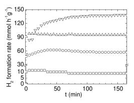
**Fig. 4.** Hydrogen formation rate as a function of time upon reaction of a 50:5:45 CH<sub>4</sub>:H<sub>2</sub>O:N<sub>2</sub> mixture over LBTss ( $\square$ ), LBTCss ( $\nabla$ ), LBTMss ( $\bigcirc$ ), and LBTCM ( $\triangle$ ) samples. T = 900 °C, 20 mg sample, total flow rate = 6.2 L h<sup>-1</sup>.
