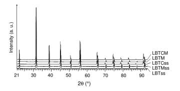
$\textbf{Fig. 1.} \ Powder\ XRD\ patterns\ of\ LBTss,\ LBTMss,\ LBTCss,\ LBTM,\ and\ LBTCM\ after\ synthesis\ in\ air.$
