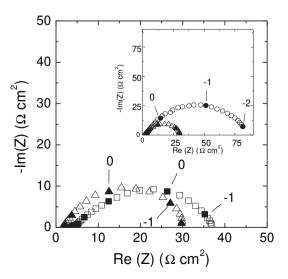
**Fig. 7.** Complex impedance spectra for LBTss ( $\Delta$ ) and LBTCss ( $\square$ ) collected on symmetrical cells (including YSZ electrolyte, BIT barrier layer and material electrodes) at 900 °C in H<sub>2</sub>/H<sub>2</sub>O(97/3). In inset: impedance spectra of LBTss at 900 °C in H<sub>2</sub>/H<sub>2</sub>O(97/3) ( $\Delta$ ) and Ar/H<sub>2</sub>/H<sub>2</sub>O(95/2/3) ( $\bigcirc$ ). Closed symbols and numbers indicate selected values of frequency (log<sub>10</sub> scale).
