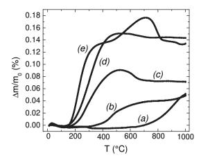
**Fig. 3.** TGA curves in air for (a) LBTss, (b) LBTCss, (c) LBTMss, (d) LBTM, and (e) LBTCM after synthesis and reduction at 900 °C for 48 h in Ar/H<sub>2</sub>(98/2).
