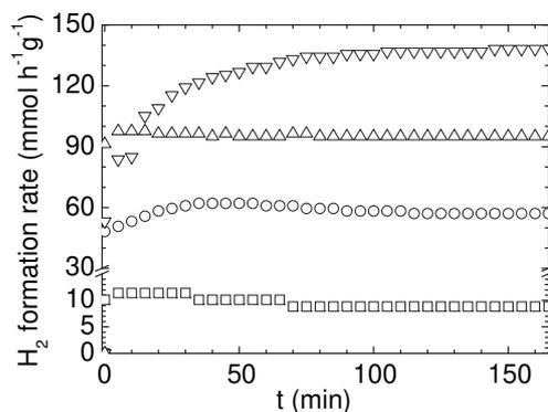
**Fig. 4.** Hydrogen formation rate as a function of time upon reaction of a 50:5:45 CH<sub>4</sub>:H<sub>2</sub>O:N<sub>2</sub> mixture over LBTss (□), LBTcSs (▽), LBTMss (○), and LBTcM (△) samples.  $T = 900$  °C, 20 mg sample, total flow rate = 6.2 L h<sup>-1</sup>.
