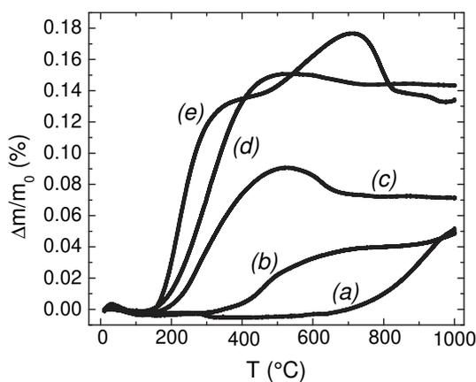
**Fig. 3.** TGA curves in air for (a) LBTss, (b) LBTcSs, (c) LBTMss, (d) LBTM, and (e) LBTcM after synthesis and reduction at 900 °C for 48 h in Ar/H<sub>2</sub>(98/2).
