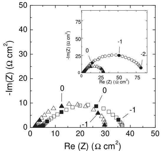
**Fig. 7.** Complex impedance spectra for LBTss (Δ) and LBTCSs (□) collected on symmetrical cells (including YSZ electrolyte, BIT barrier layer and material electrodes) at 900 °C in H<sub>2</sub>/H<sub>2</sub>O(97/3). In inset: impedance spectra of LBTss at 900 °C in H<sub>2</sub>/H<sub>2</sub>O(97/3) (Δ) and Ar/H<sub>2</sub>/H<sub>2</sub>O(95/2/3) (○). Closed symbols and numbers indicate selected values of frequency (log<sub>10</sub> scale).
