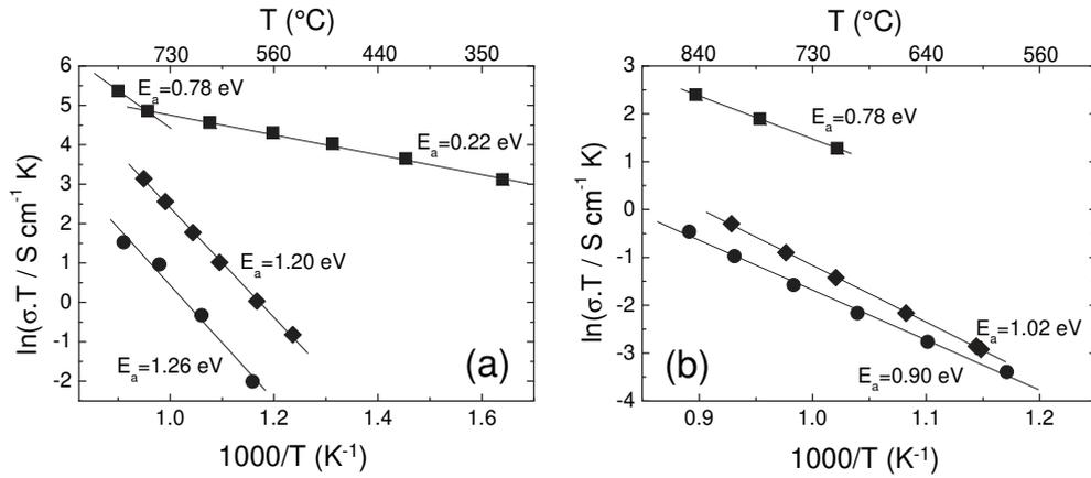
**Fig. 5.** Arrhenius plot of electrical conductivity for (◆) LBTM, (●) LBTMs, and (■) LBTCSs measured (a) in Ar/H<sub>2</sub>(98/2) and (b) in air. Activation energy values ( $E_a$ ) were determined from the Arrhenius law.
