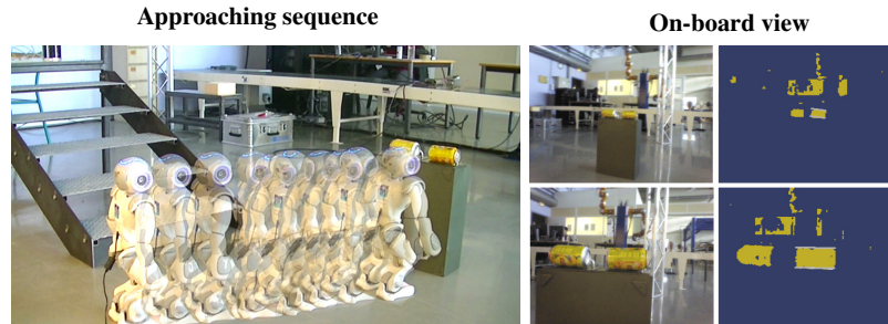
Fig. 8: Experimental task. The trajectory followed is shown on the left, whereas some on-board views and their corresponding color saliency are shown on the right.
