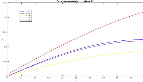
FIGURE 7. Total density for different values of  $\varepsilon$ .  $\varepsilon = 0$  corresponds to the limiting nonlinear diffusion model (1.4).
