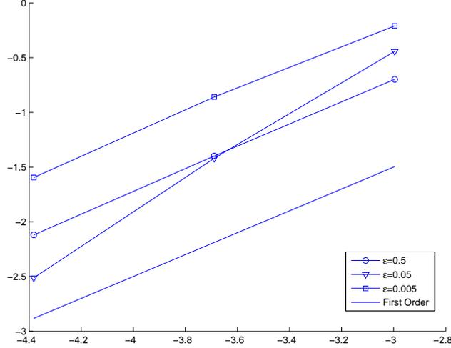
FIGURE 1. Convergence order with respect to  $\Delta x$ . Here the log-log plot of the mesh sizes with respect to the  $L^1$  norm of the probability density error in all directions is displayed. The mesh sizes are  $1/20$ ,  $1/40$ ,  $1/80$ ,  $1/160$  and  $e_{\Delta x} := \max_{x \in (-1,1)} \|f_{\Delta x}(x, t) - f_{2\Delta x}(x, t)\|_1$  are plotted for different  $\varepsilon$ .
