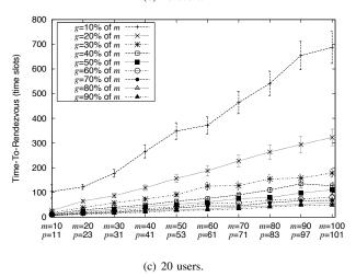
Fig. 4. Average TTR for asymmetric two, 10 and 20 users executing the jump-stay rendezvous algorithm in 10 to 100-channel scenarios obtained with the OMNeT++ simulations.
