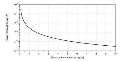
Fig. 1. At five meters, an EPC Gen2 tag receives around 100  $\mu W$  from the reader
