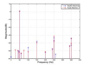
Fig. 5. The frequency estimations for a healthy and faulty induction motors are obtained with the Root-MUSIC for L=20. The model order estimation is obtained thanks to two proposed information criteria (AIC and MDL).
