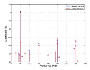
Fig. 6. The frequency estimations for a healthy and faulty induction motors are obtained with the ESPRIT for L=20. The model order estimation is obtained thanks to two proposed information criteria (AIC and MDL).
