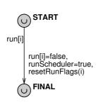
Seq(c1,c2): suppose a1 and a2 are the automata for c1 and c2 respectively, add an edge from final1 to start2, start1 is the start state, final2 is the final state. The edge has a guard checking run[i] and an update setting run[j  $\neq$  i] to false.
