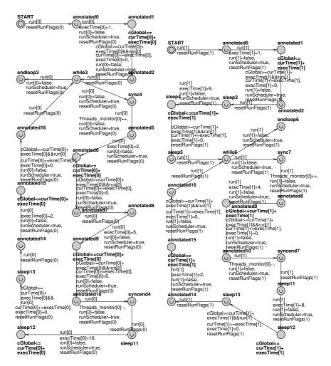
**Fig. 3.** Generated automata for threads t1 and t2.
