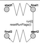
Cond(e,c1,c2): suppose a1 and a2 are the automata for c1 and c2 respectively, add two urgent states START and FINAL, which are the start and final states of the new automaton, and edges from START to start1 and start2, from final1 and final2 to FINAL. The edges from START to start1, start2 have guards checking run[i] and updates resetting run[i] to false,
