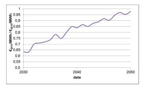
Fig. 2. Ratio of the nuclear annual levelized cost of electricity between the "prog." scenario and the "40 yrs" scenario (50% nuclear penetration),  $\varepsilon_{2010}/MWh / \varepsilon_{2010}/MWh$ , own calculus
