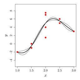
Figure 2: Kriging mean  $m^{PI}(x)$  (thick line) and confidence intervals  $m^{PI}(x) \pm 2\sqrt{v^{PI}(x)}$  (thin lines). Kriging mean using pseudoinverse goes exactly through the average of the outputs. The observed values are  $\mathbf{y} = (-2, -1, 0, 1.5, 4, 7, 7.5, 6, 5, 3)^{\top}$ .  $m^{PI}(1.5) = -0.5$ ,  $m^{PI}(2) = 5$ , and  $m^{PI}(2.5) = 5.5$ . Note that  $v^{PI}$  is zero at redundant points.
