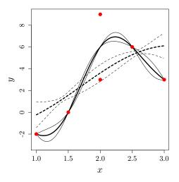
Figure 7: Effect of the tolerance  $\tau$  on the kriging model regularized by PI. Dashed line,  $\tau=1$ ; continuous line,  $\tau=10^{-3}$ . Except for  $\tau$ , the setting is the same as that of Figure 6. When the tolerance is large ( $\tau=1$ ), the 5th eigenvector is deleted from the effective image space of  $\bf C$  in addition to the 6th eigenvector, and the PI regularized model is no longer interpolating. Same  $\bf X$  and  $\bf y$  as Figure 4.
