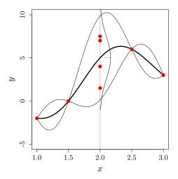
Figure 8: Distribution-wise GP,  $m^{Dist}(x)$  (thick line)  $\pm 2\sqrt{v^{Dist}(x)}$  (thin lines). At the redundant point x=2, the outputs are 1.5, 4, 7 and 7.5. The mean of the distribution-wise GP passes through the average of outputs. Contrarily to PI (cf. Figure 2), distribution-wise GP preserves the empirical variance: the kriging variance at x=2 is equal to  $s_{x=2}^2=5.87$ .
