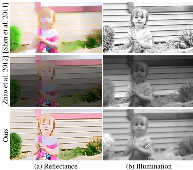
Figure 5: We compare our technique (third row) to the decompositions of Shen et al. [2011] (first row) and Zhao et al. [2012] (second row). Shen et al. has brushes and takes 6 min. while Zhao et al. is automatic and takes 6 s. Our method takes 0.5 s per frame, and provides a more satisfactory decomposition for our applications.
