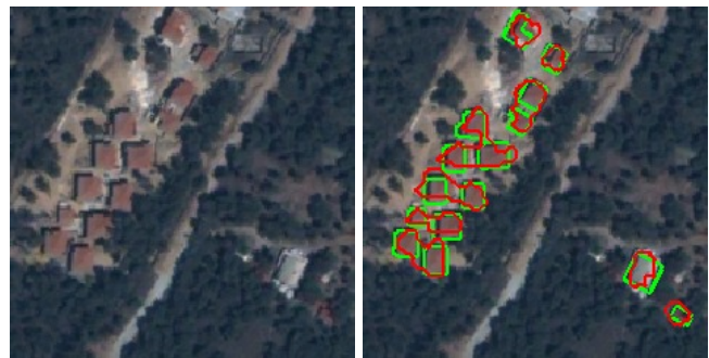
Fig. 1. Automated building detection from very high resolution multispectral data. The developed algorithm managed to detect efficiently scene’s buildings. The ground truth data are shown with a green color, while the detected buildings with red.
