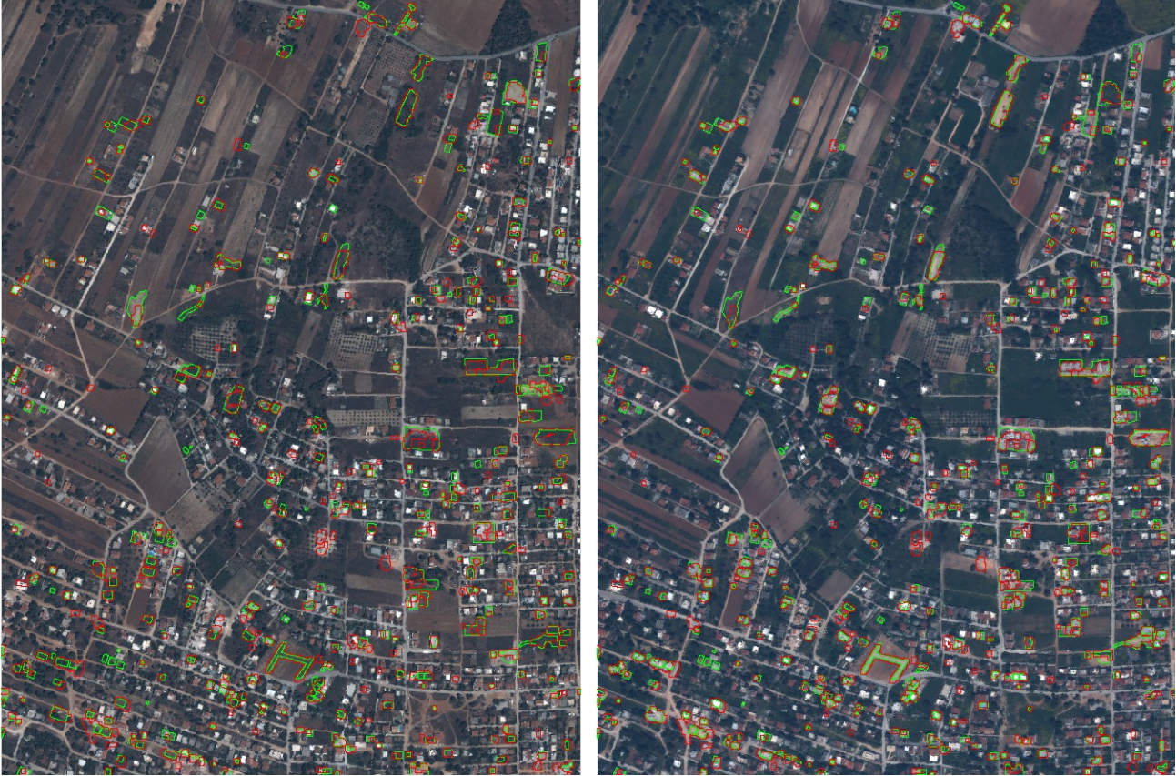
Figure 3. Experimental results after the application of the developed method. The detected changes are shown with red color and the ground truth with green. Both are superimposed to the very high resolution satellite images acquired in 2006 (left) and 2011 (right).
