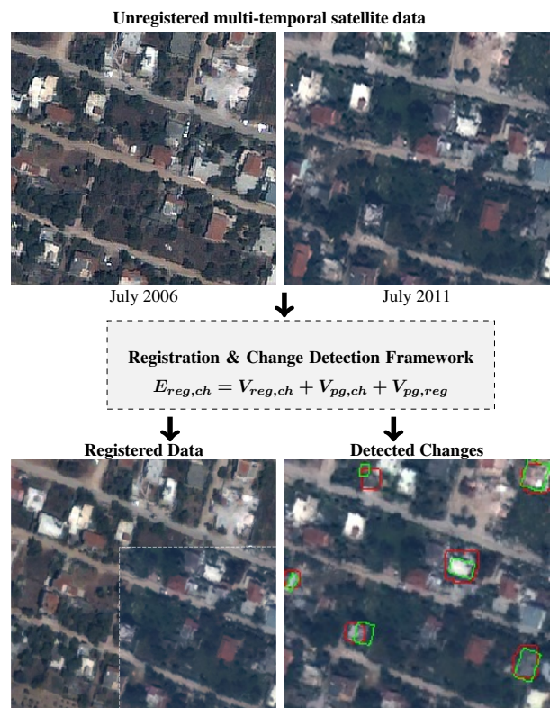
Figure 1. The developed framework addresses simultaneously the registration and change detection tasks.
