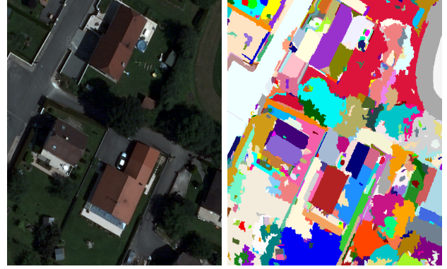
Figure 3. Example of segmentation result using Statistical Region Merging (SRM) method. From left to right: Original image and its SRM segmentation result.
