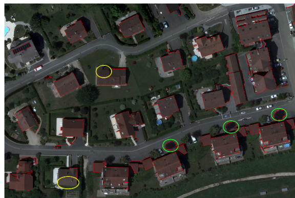
Figure 5. Examples of some building parts that have not been extracted (yellow ellipses) and some false detections (green ellipses)
