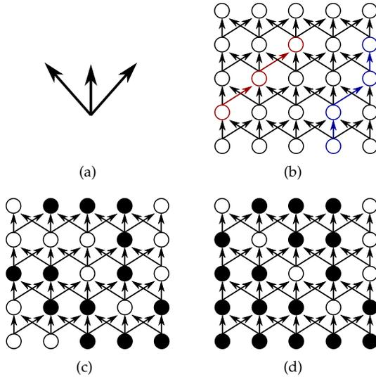
Fig. 3. (a) An example of adjacency relation  $\rightarrow$ . (b–d) The connectivity  $\Gamma$  which is a periodic repetition of (a) over  $X$ . (b) A path of length 3 (resp. 4) is depicted in red (resp. blue). (c) A binary image defined on  $X$ . (d) The result of a path opening of length 4 on the image of (c).
