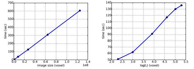
Fig. 10. Computational cost of RORPO, with respect to  $|\Omega|$  (left) and  $L$  (right, log scale).
