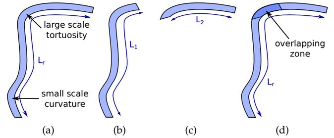
Fig. 8. The path length also depends on the scale of the curvature. (a) A thin structure of length  $L_r$  presenting small-scale and large-scale curvature. (b) A path length of length  $L_1 < L_r$  along one orientation detects a first part of the structure. (c) A path length of length  $L_2 < L_r$  along another orientation detects a second part of the structure. (d) The two detected parts overlap.
