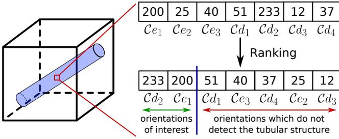
Fig. 6. At each point of an image (red square), 7 path opening responses  $A_L^\Gamma(I(x))$ , associated to each orientation  $C_*$ , are computed (top right values). After ranking, the orientations of interest are the first one, two or three orientations.
