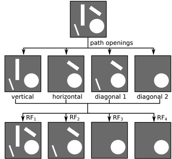
Fig. 5. 2D illustration of filter response ranking. A structure present in one orientation (the vertical line) remains in  $RF_1$ ; structures present in two orientations (the oblique lines) remain in  $RF_1$  and  $RF_2$ ; the disc is present in all the orientations and thus remains in all the  $RF$ s.
