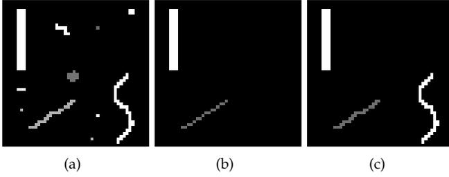
Fig. 2. Comparison on image (a) of a classical path opening (b) and a path opening (c) with the same SE length of 10 pixels. The bottom right line is globally vertical but presents local tortuosity. Only the path opening is able to detect such structure.
